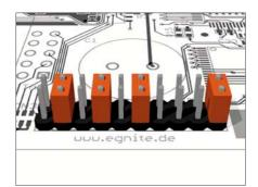
JP5 As an alternative, the Ethernut is able to program its own CPLD. The required jumper configuration is shown on the left.
