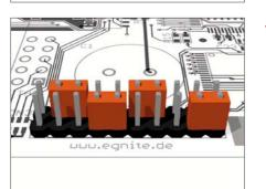
JP5 Routing the JTAG interface to the CPLD is provided by shortening pins 1 and 3, 4 and 6, 7 and 8 as well as pins 9 and 10. However, you need a special Xilinx adapter for programming the CPLD via JTAG.
