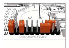
JP5 Jumper JP5 routes the JTAG signals to the AT91R40008, if pins 1 and 2 and pins 5 and 6 are shortened.
