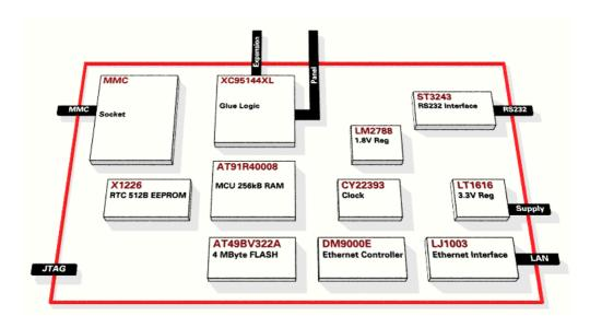
The microcontroller provides two UART channels, which are routed to the onboard RS-232 level shifters.
